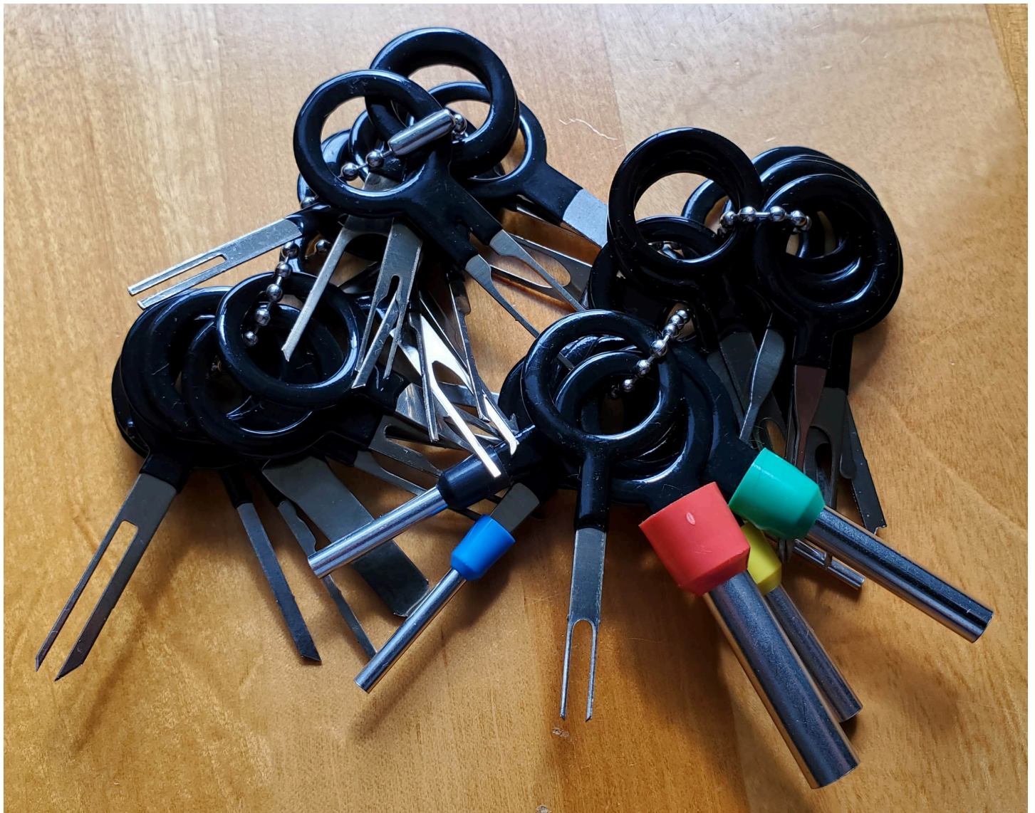
Tools for extracting individual wires and clips from large plug harnesses - fun indeed
